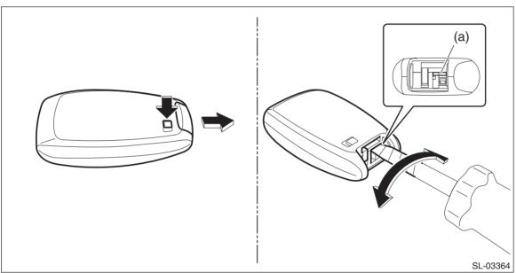
3) Remove the battery (a) from the case.
